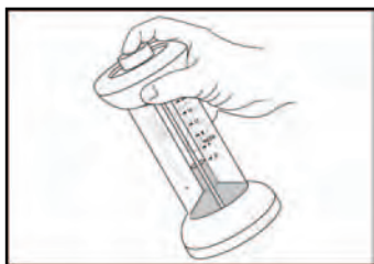
Figure 3. Venting FYRITE® to Atmosphere at 45° Angle
